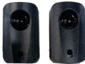
AGS-SBS100 Power supply : 12V~24V AC/DC Max. Range: 15M Input: RX 15mA, TX 30mA Infrared frequency: 1.92KH Wave length: 940nm Relay output: 1A max 36V
