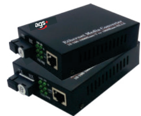
AGS-MCBI3512-20 / AGS-MCBI5312-20 10/100/1000M SM Single Fiber, T1310/1550nm, SC, 20Km
