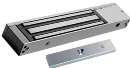
AGS-SD600LB Holding Force : 280KG (600Lbs) Single Door Power : 12 to 24 VDC Body Type : Zinc
